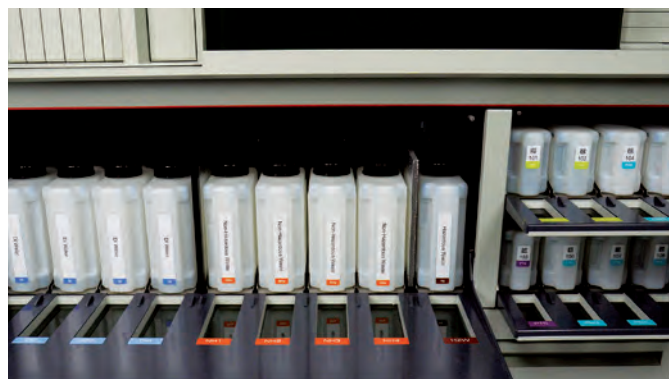
Figure 9.10 More onboard capacity for reagents and bulk fluid bottles can reduce hands-on time due to little or no reagent handling during the day.
