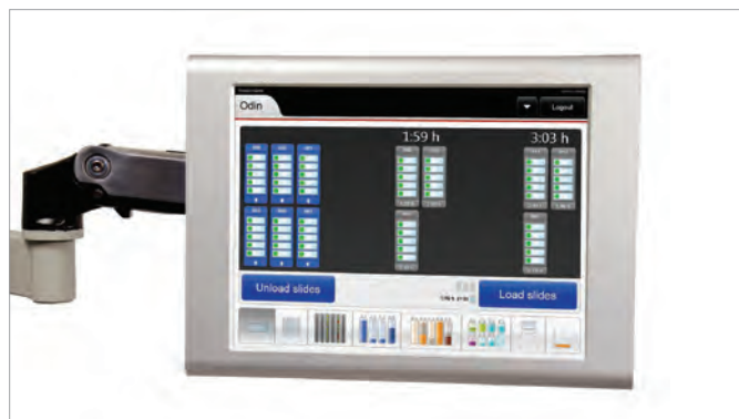
Figure 9.8 The scheduler software organizes the sequence of all individual steps an instrument must perform from start to end of the staining process for the given load of slides. For some instruments, the scheduler also calculates when slides will be completed.
